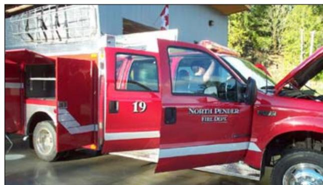
Truck 19 has a Ford, F-550 super-duty chassis, an optional four-wheel-drive and is powered by a 7.3 liter diesel turbo-charged engine. The truck options were specified with the island roads, driveways and extreme road conditions in mind.
