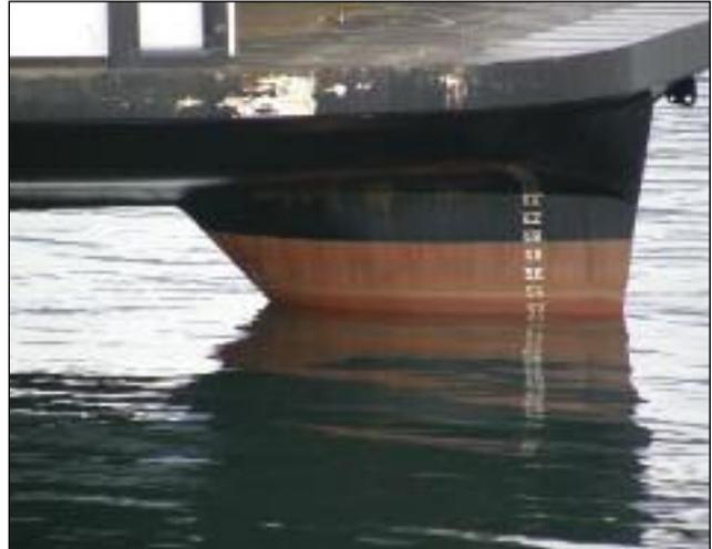
One of the rudders of the *Coastal Celebration*. The vessel is berthed, unloaded, and the propellers are stationary. Note the draft markings.
